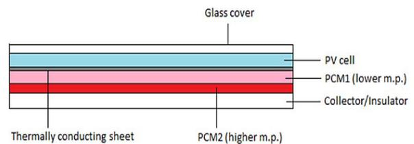
**Fig. 8** Multi PCM layers using for efficient cooling [64].
