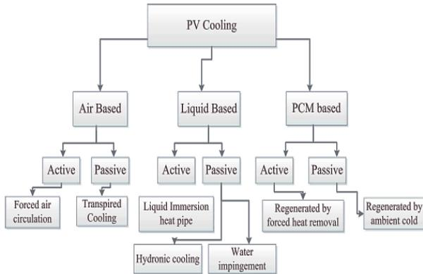
**Fig. 3** Commonly utilized PV cooling method [31].
