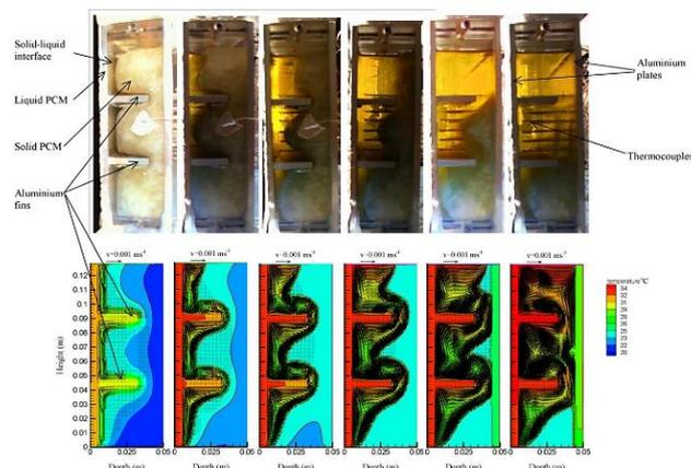
**Fig. 6** Photovoltaic image for a PV-PCM unit using fins throughout the PCM melting process [44].
