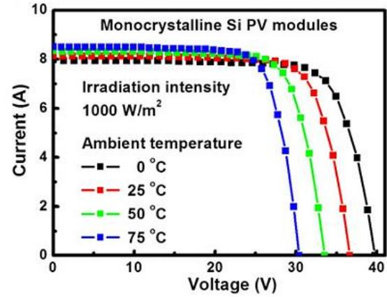
**Fig. 2** Characteristics of current-voltage at 1000 W/m<sup>2</sup> solar intensity [28].
