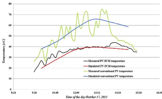
**Fig. 7** Measured and simulated temperatures for PV-PCM and standard PV panel [46].
