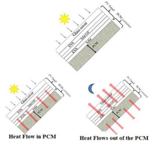
**Fig. 4** Working principles of the basic PV-PCM system [38].
