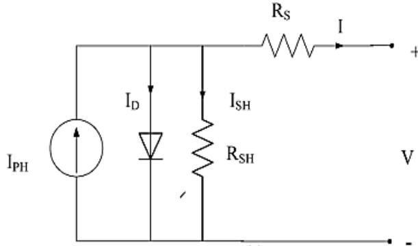
**Fig. 1** A single PV cell circuit [23].
