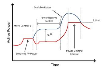
Fig. 1 Three different active power control schemes action times
