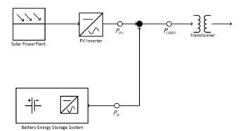
Fig. 2 Schematic of a PV power plant generation and a connected BESS to grid
