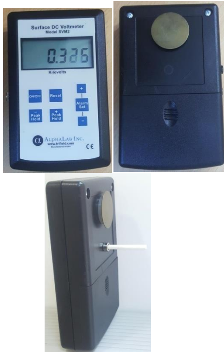
Fig. 1 Electric static charge (voltage) measuring device.
