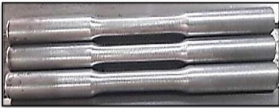
Fig. 4 Dog bone specimens of the base metal
