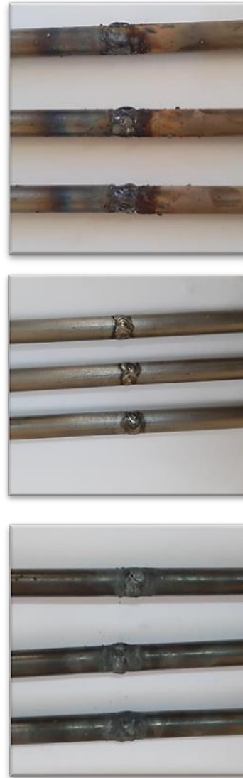
Fig. 2 (Top to bottom) SMAW, MIG, and OAW joints
