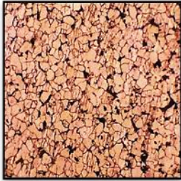
Fig. 1 Microstructure of the base metal with estimated (0.25-0.3%C) ,(X160).
