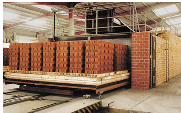
Figure 10. Tunnel kiln for firing bricks.
