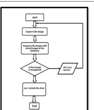
Fig.1. Flowchart for Face Recognition System
