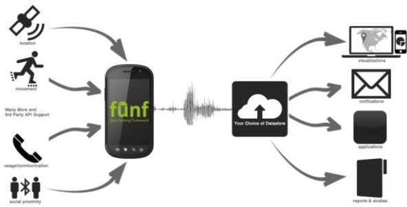
Fig. 2. A snippet of the Funf framework, [9]. It shows the sensors on an Android device that can collect data, such as the GPS sensor, the accelerometer, or the microphone. The data collected is stored in a local memory or on a server. The Funf framework supports a variety of data storage options, including SQLite, CouchDB, and Amazon.
