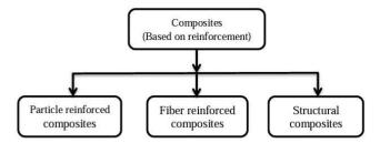
Fig. 1 composites types according to kind of reinforcement [18].
