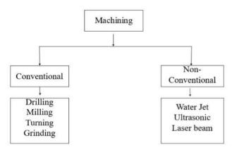
Fig. 2. Machining process types for various materials [56].
