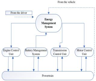
Fig. 4: control scheme of an HEV.
