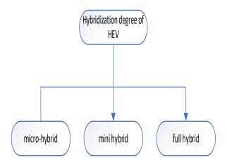
Fig. 2: Classification of HEV based upon hybridization.
