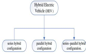
Fig. 1: Classification based upon the structure of HEV.
