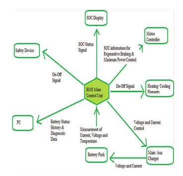
Fig. 3: Functions of battery management system.
